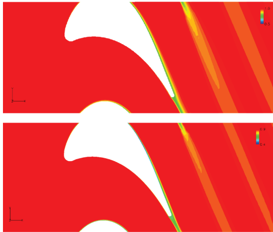
Fig.6: Comparison between BOXER (above) & FLUENT (below) : scaled entropy – range 0.5 to 1.0
